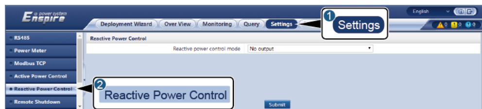
Figure 8-2 Reactive power control
