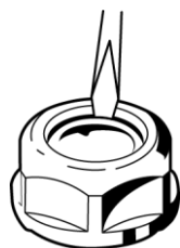
Figure 5-7 Stripping a seal ring
